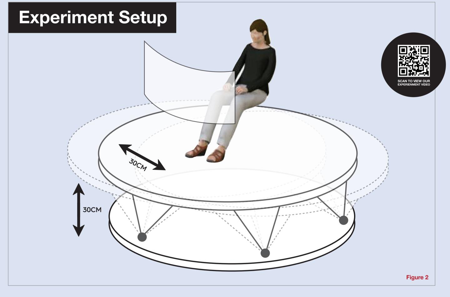
There are 3 conditions, where the motion platform is stationary, moving in the same direction as the motion on the display, or in the opposite direction. A staircase procedure is applied (6 turning points where the average of the last 5 is calculated as the threshold value (for an example see Figure 3). See Figure 4 for one observer, where we highlight the 1 deg/s performance for the three conditions.
